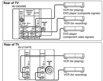
When you use VIDEO-1 INPUT, you should choose to connect S-VIDEO or video input. If S-VIDEO connector and video input are connected at the same time, no picture display on the screen and the message "PLEASE DISCONNECT VIDEO-1 CABLE!" appears. In this case, you should disconnect either S-VIDEO or video input.
